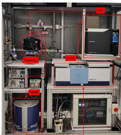
Figure 1: The operando miniplant, containing a GC, NMR, and FTIR.
