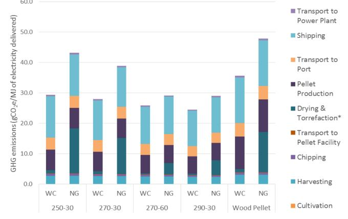
Greenhouse gas (GHG) emissions per MJ of electricity delivered for 4 different torrefied pellets (TP) and conventional wood pellets (WP) using wood chips (WC) or natural gas (NG) as utility fuel. \*For wood pellets = drying only
